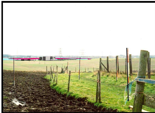
Figure 1 Aligning model in photograph to reference points (surveyor's rods)
